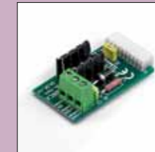
DA.RB Battery charger card for DA.S04
